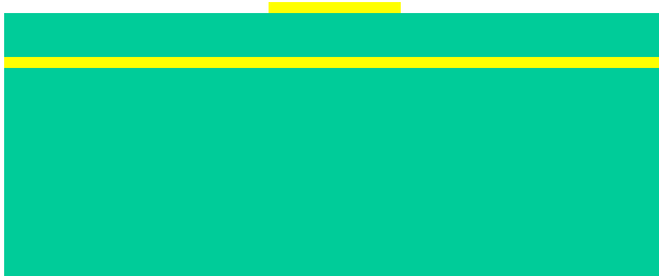
Figure 1.4. Photolithography and RIE are used to transfer the pattern of the first level mask (BRIDGE) on to the oxide layer.
