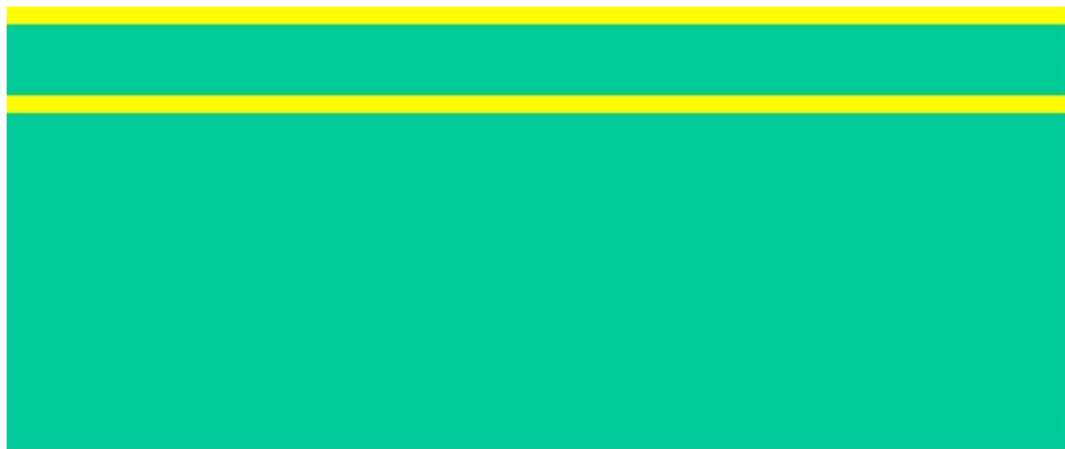
Figure 1.3. A layer of PECVD silicon dioxide is deposited on top of the silicon device layer at a temperature of 200 ^{\circ}\text{C} . The PECVD silicon dioxide layer serves subsequently as a releasable insulator structural layer.
