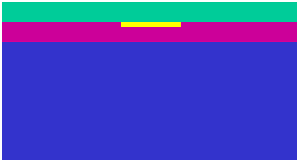
Figure 1.7. The silicon substrate and the BOX layer of the SOI wafer are removed.
