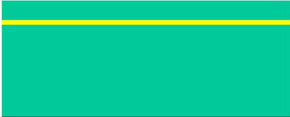
Figure 1.2. The starting material is a SOI wafer with a 20 \mu\text{m} silicon device layer, a 0.5 \mu\text{m} silicon dioxide layer, and a 500 \mu\text{m} silicon substrate layer.
